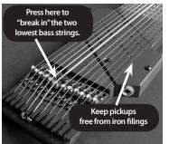
**CLEANING THE PICKUPS:** Minute iron particles may cling to the tops of the magnetic pickups. Under the 1st and 2nd strings, where the pickups are set high for volume, such iron bits might touch the strings and distort the sound. These ferrous bits can be removed by touching them with any pointed iron or steel object and drawing them away (the accessory 1/16" hex wrench is recommended for this use).
